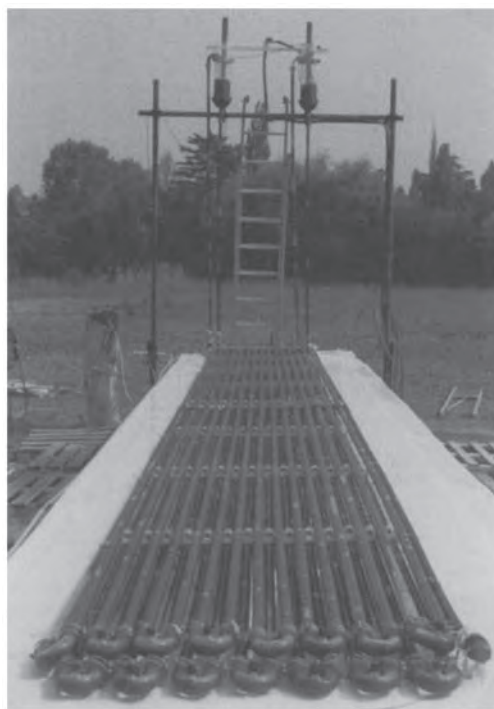
Figure 6.2 General view of a two-plane air-lift tubular bioreactor made of Plexiglas® tubes 2.6 cm i.d. devised by Centro di Studio dei Microrganismi Autotrofi, CNR, Florence, Italy.
