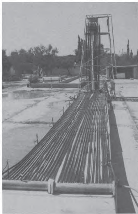
Figure 6.3 A tubular bioreactor installed at Microalgal Biotechnology Laboratory, Sede-Boker, Israel. (From Richmond et al., 1993, with permission.)
