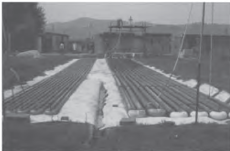
Figure 6.1 General view of tubular bioreactors made of Plexiglas® tubes 7.4 cm and 13.1 cm i.d. operated by Centra di Studio dei Microrganismi Autotrofi, CNR, Florence, Italy.
